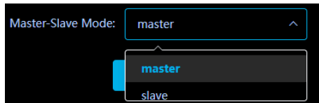
Fig 31 Set the RS485 master/slave mode
