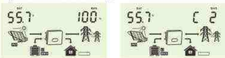
Battery SOC is 100%
