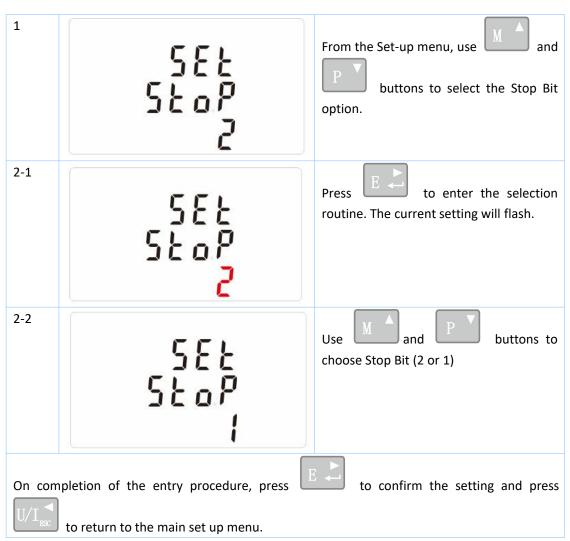
Note: Default is 1, and only when the parity is NONE that the stop bit can be changed to 2.
