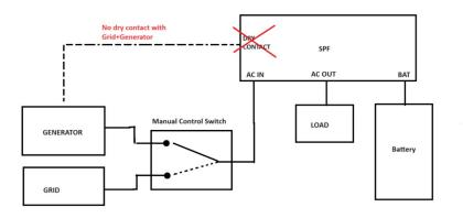
Dry contacts cannot be used when both generator and grid are connected to the inverter, this may cause generator to turn on without being connected.
