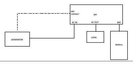
If dry contact is to be used, the generator must be compatible with dry contact functions, SPF must be upgraded to newest versions of firmware.
